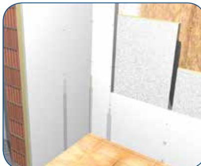
Available also is the **STIFERITE AV** series panels, bonded with facers of embossed aluminium on one side and saturated fibre glass on the other.
